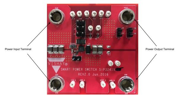
Fig. 1 - SiP32419EVB, SiP32429EVB Evaluation Board Rev. 2.0
