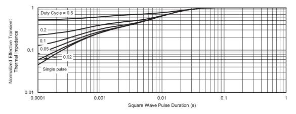
Normalized Thermal Transient Impedance, Junction-to-Case
