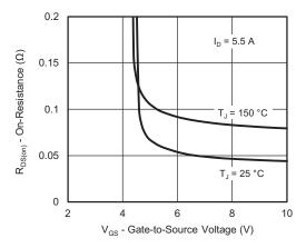
On-Resistance vs. Gate-to-Source Voltage
