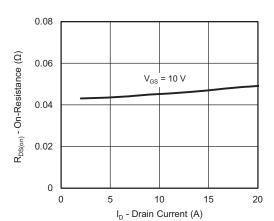
On-Resistance vs. Drain Current and Gate Voltage
