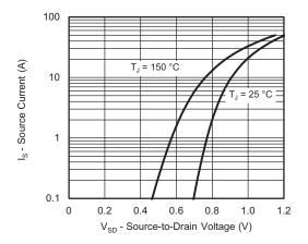
Source-Drain Diode Forward Voltage
