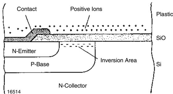
Fig. 3 - Function of Parasitic Field Effect Transistor as a Result of Failure (Latch-up) in the Phototransistor of Couplers
