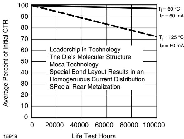
Fig. 4 - Degradation under Typical Operating Conditions
