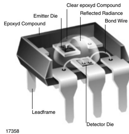
Fig. 1 - Coplanar Construction Principle
