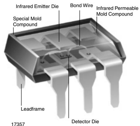
Fig. 2 - Face to Face Construction Principle
