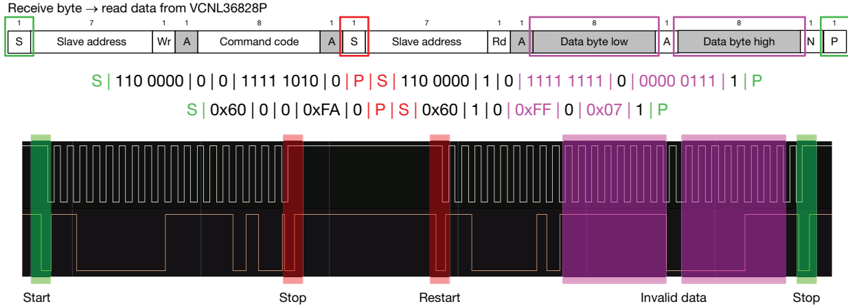
Fig. 41 - The Incorrect I 2 C Read When Reading the Register VCNL36828P_ID With Both Stop and Restart Conditions
