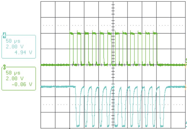
**Green waveform:** optical input signal to the photodiode that is connected to the amplifier circuit.
