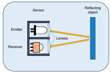
Fig. 9 - Sensor Example With Plano-Convex Lenses
