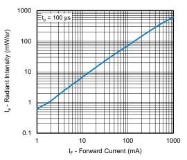
Fig. 6 - TSAL6200 Emitter Intensity vs. Forward Current
