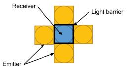
Fig. 8 - Sensor Example With Four Emitters Surrounding one Receiver Separated With an Optical Barrier
