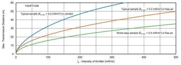
Fig. 3 - Comparison of the Transmission Distance in Free Air and a Long Corridor
