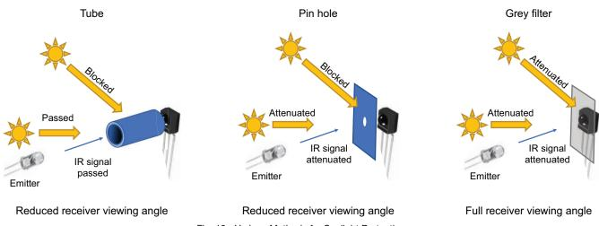
Fig. 12 - Various Methods for Sunlight Protection Left: Tube, Middle: Pinhole, Right: Grey Filter
