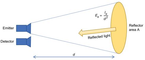
Fig. 4 - Illustration of the Light Path in a Reflective Sensor
