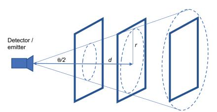
Fig. 5 - Illustration of how the Fraction of the Radiating Reflector Area Seen by the Detector Increases With the Distance *d* Until the Receiver's Field of View Becomes Larger Than the Reflector Size
