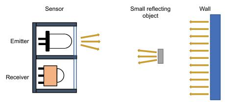
Fig. 7 - Detection of a Small Object in Front of a Large Strongly Reflecting Wall
