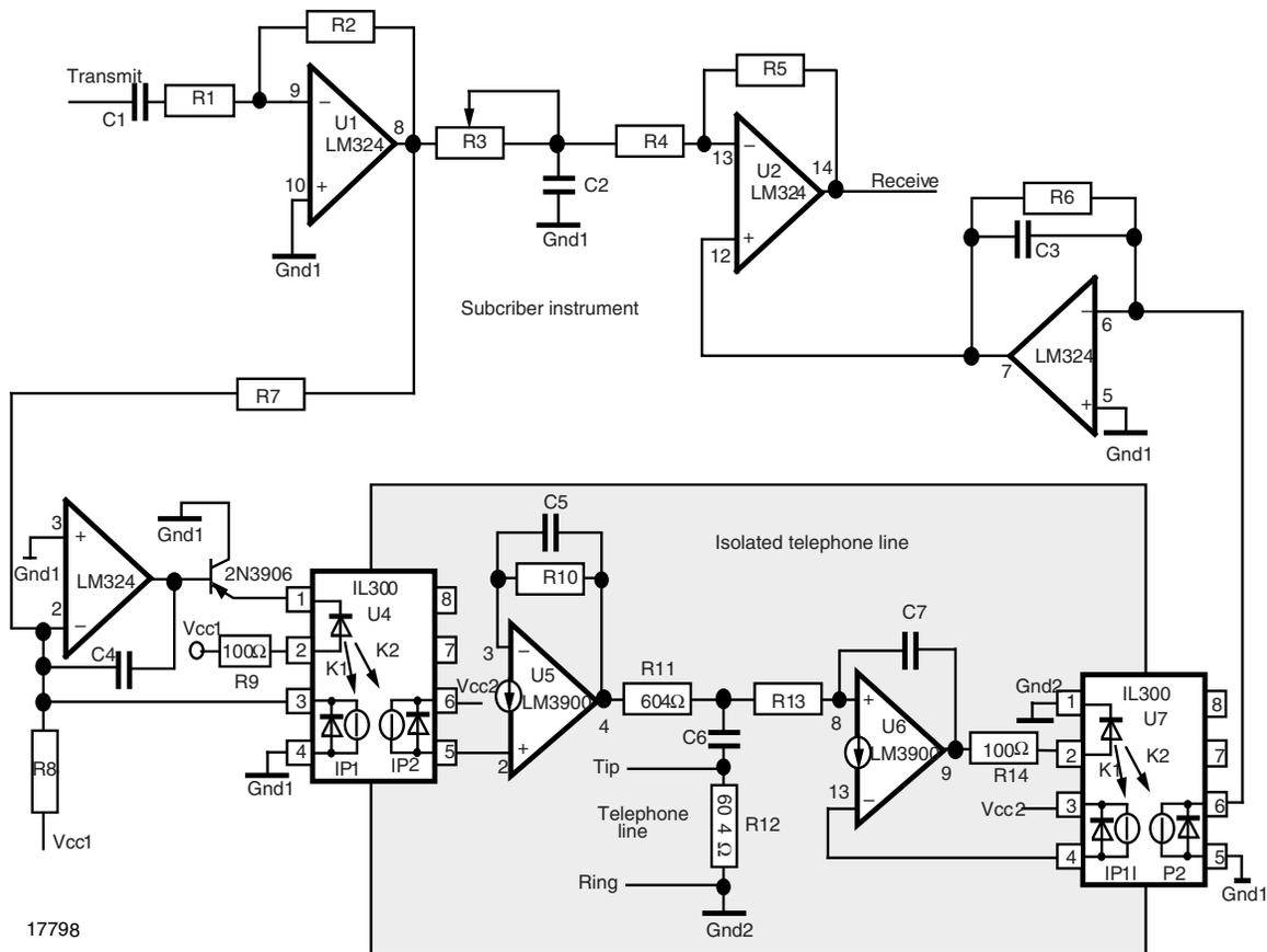
Fig. 5 - 2 to 4 Wire Optically Coupled Hybrid Norton/Thevenin Amplifier
