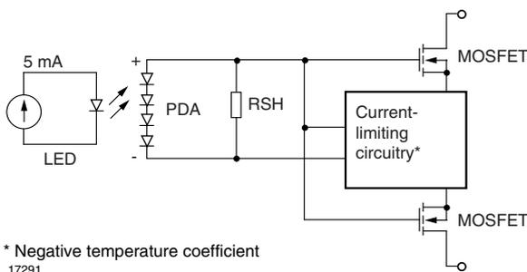
Fig. 1 - Current-Limit SSR Schematic
