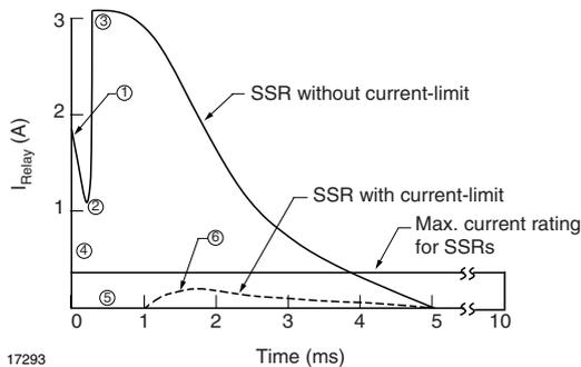
Fig. 2 - Anatomy of a Current-Limit SSR During Lightning
