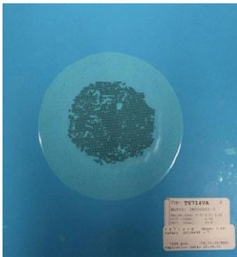
Fig. 1 - Sawn Dice on Loose Foil
