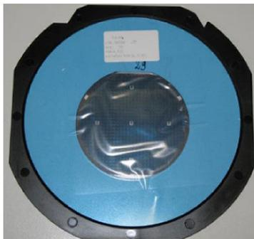
Fig. 2 - Sawn Dice on Disco Frame
