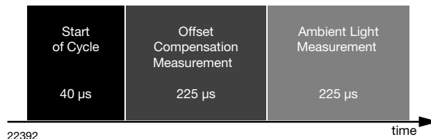
Fig. 16 - Timing Diagram for Individual Measurement Cycle
