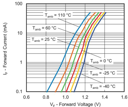
Fig. 2 - Forward Current vs. Forward Voltage
