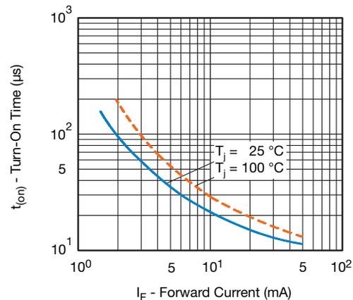
Fig. 1 - Turn-On Time vs. Forward Current
