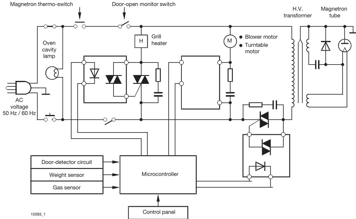
Fig. 34 - Microwave Oven With Grill Example
