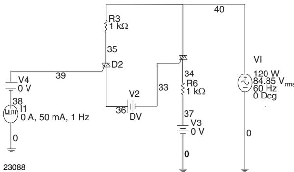
Fig. 24 - In Depth TRIAC Driver Model
