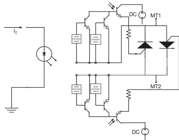
Fig. 9 - Phototriac Functional Diagram
