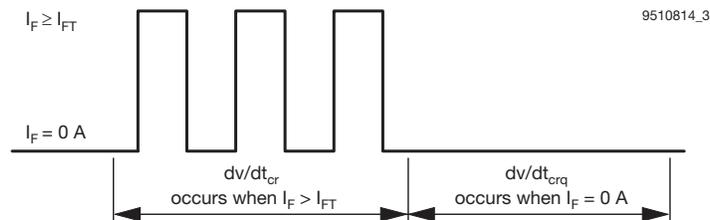
$dv/dt_{cr}$  Highest value of the "rate of rise of off-state voltage" which does not cause any switching from the off-state to the on-state
