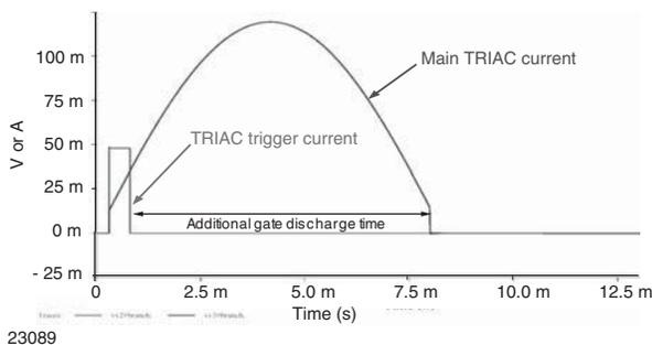
Fig. 25 - TRIAC Driver Waveforms
