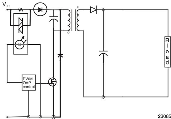
Fig. 20 - Inrush Limit Bypass Application
