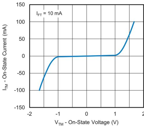
Fig. 26 - Characteristics Curve of an Phototriac
