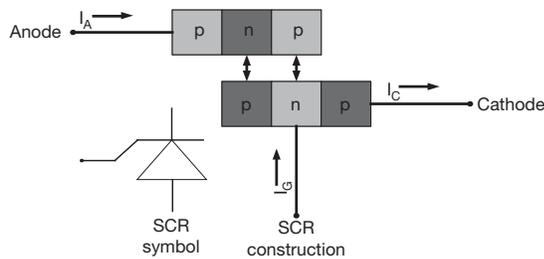
Fig. 7 - SCR Construction
