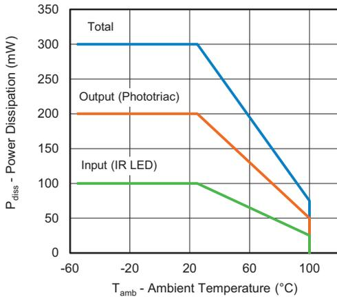
Fig. 30 - Allowable Dissipated Power
