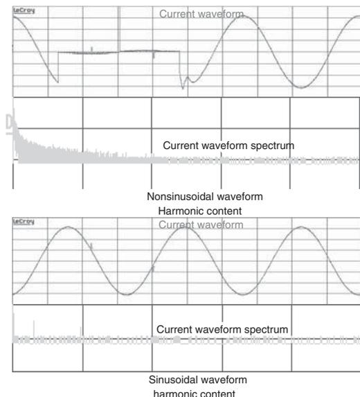
Fig. 12 - Harmonic Content of Non-Sinusoidal Current Waveforms
