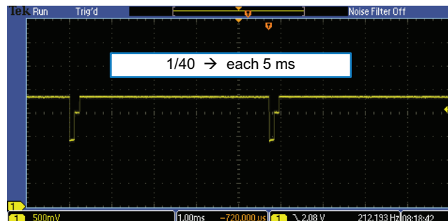
Fig. 15 - Proximity Measurements with PS_Duty = 1/40
