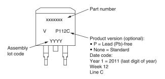
Example: This is a xxxxxxx with assembly lot code YYYY, assembled on WW 12, 2011 in the assembly line "C"
