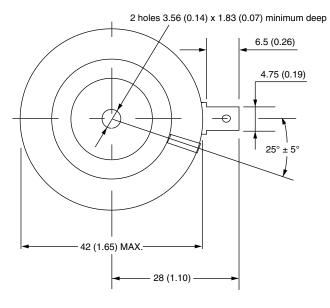
Quote between upper and lower pole pieces has to be considered after application of mounting force (see thermal and mechanical specification)
