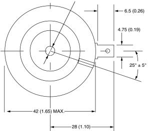
Quote between upper and lower pole pieces has to be considered after application of mounting force (see thermal and mechanical specification)
