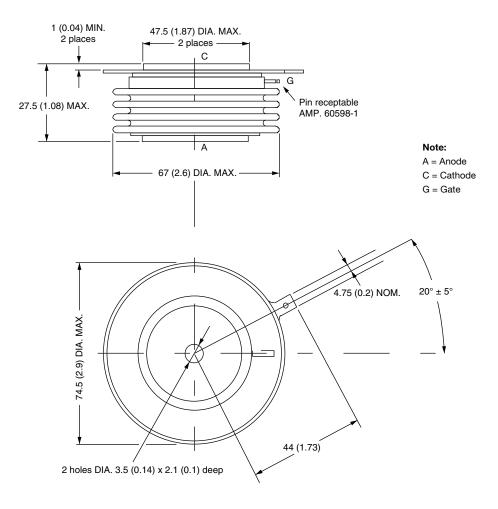
Quote between upper and lower pole pieces has to be considered after application of mounting force (see thermal and mechanical specification)
