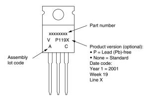
Example: This is a xxxxxxxx with assembly lot code AC, assembled on WW 19, 2001 in the assembly line "X"
