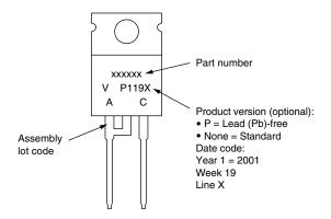
Example: This is a xxxxxx with assembly lot code AC, assembled on WW 19, 2001 in the assembly line "X"
