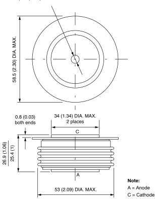
Quote between upper and lower pole pieces has to be considered after application of mounting force (see Thermal and Mechanical Specifications)
