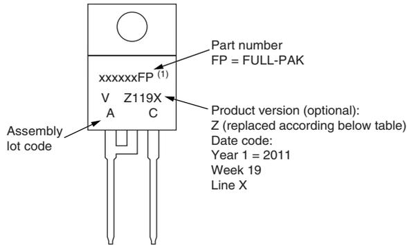
Example: This is a xxxxxxFP<sup>(1)</sup> with assembly lot code AC, assembled on WW 19, 2011 in the assembly line "X"
