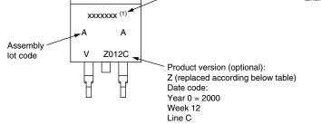
assembly lot code YYYY, assembled on WW 12, 2000 in the assembly line "C"
