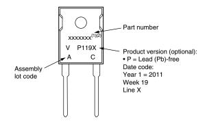
Example: This is a xxxxxx with assembly lot code AC, assembled on WW 19, 2011 in the assembly line "X"
