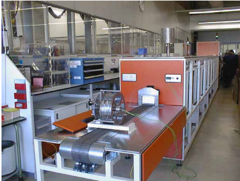
Fig. 5: Furnace prototype. In the foreground the conveying belt, which transports the diodes in the carbon container, is visible. On the top (right hand side) of the picture the safety contrivance, which burns emergent H 2 gas to avoid dangerous concentrations of H 2 in the production hall, is shown.
