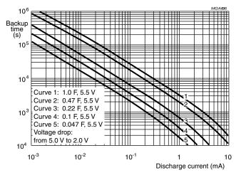
Fig. 9 - Typical backup time as a function of discharge current
