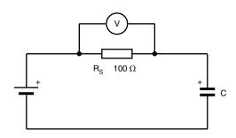
Fig. 6 - Test circuit for leakage current
