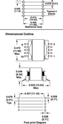
**NOTE:** Pad layout guidelines per MIL-STD-275E (printed wiring for electronic equipment). Tolerances:  $xx \pm 0.01^{"}$  [± 0.25 mm];  $xxx \pm 0.005^{"}$  [± 0.12 mm]
