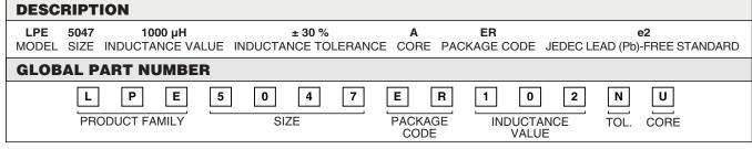
NOTE Series is also available with SnPb terminations by using package code RY for tape and reel (in place of ER) or SM for bulk (in place of EB).
