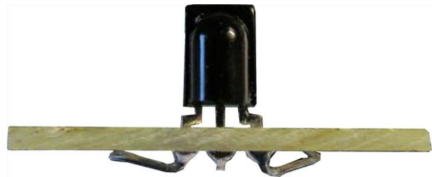
Fig. 2 - Example: Minicast Receiver Mounted on PCB
