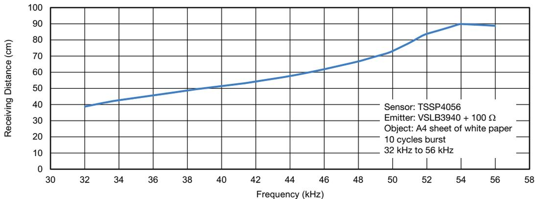
Fig. 5 - Receiving Distance of the TSSP Sensor Kit at Different Modulation Frequencies
