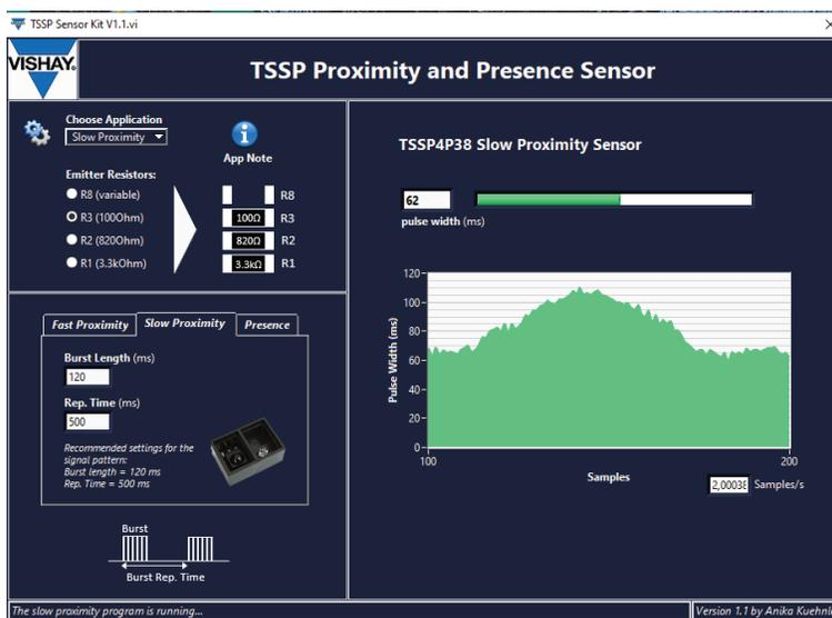
Fig. 9 - Operating Panel of the Slow Proximity Function in the TSSP Sensor Kit
