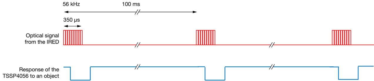
Fig. 2 - Pulsed Signal of the TSSP Presence Sensor Function in the Sensor Kit
