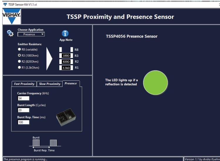
Fig. 3 - Operating Panel of the Presence Function in the TSSP Sensor Kit
