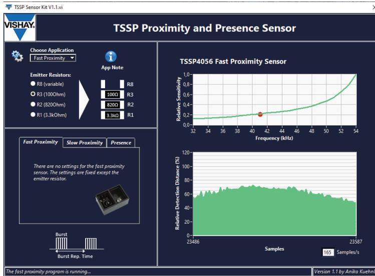
Fig. 6 - Operating Panel of the TSSP4056 Fast Proximity Function in the TSSP Sensor Kit
