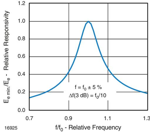
Fig. 4 - TSSP4056 Relative Responsivity vs. Relative Modulation Frequency
