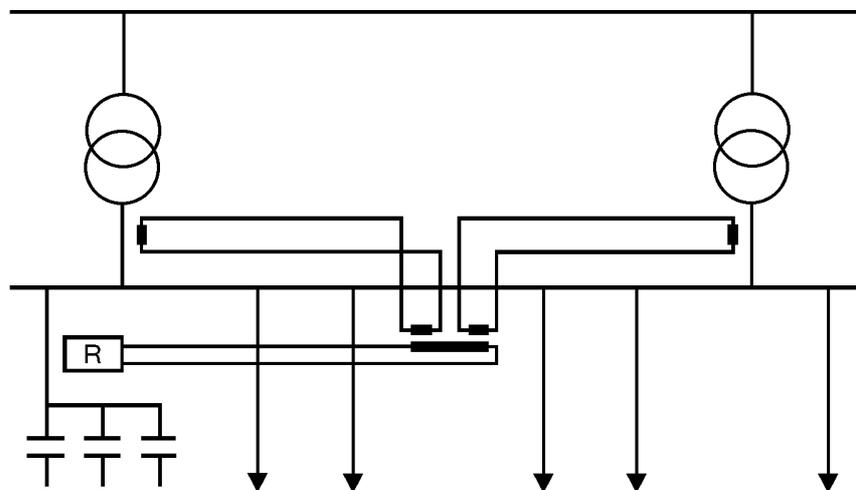
When several transformers supply one single L.V. bus bar, the individual currents shall be measured by means of current transformers and then added together via a summation current transformer. Special attention shall be given to the correct polarity because, otherwise, the current intensities of the individual transformers will subtract.
