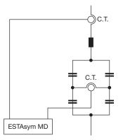
It is possible to configure the four current inputs of the ESTAsym MD for different applications. For a YY- or bridge connection, inputs 1-3 will be the three line currents, and the fourth input would be the unbalance current. It is also possible to use the first input to measure the line current and inputs 2-4 can be used for the unbalance measurements. Thus it is possible to control three individual YY or bridge connections with different unbalance settings for each bank.
