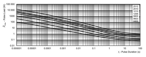
Maximum pulse load, single pulse; applicable if  $\overline{P} \rightarrow 0$  and  $n \le 1000$  and  $\hat{U} \le \hat{U}_{max}$ ; for permissible resistance change equivalent to 8000 h operation
