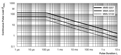
Maximum pulse load, continuous pulse; applicable if  $\bar{P} \leq P$  ( $9_{amb}$ ) and  $\hat{U} \leq \hat{U}_{max}$ ; for permissible resistance change  $\pm$  (0.5 % R + 0.01  $\Omega$ )
