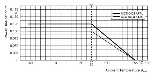
For permissible resistance change please refer to table MAXIMUM RESISTANCE CHANGE AT RATED DISSIPATION, above. **Derating - Power Mode**
