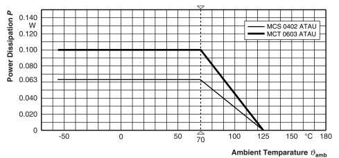
For permissible resistance change please refer to table MAXIMUM RESISTANCE CHANGE AT RATED DISSIPATION, above. **Derating - Standard Mode**
