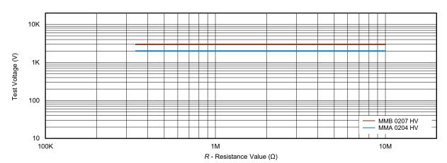
Pulse load rating in accordance with IEC 60115-1, 4.27; 10  $\mu$ s/700  $\mu$ s; 10 pulses at 1 minute intervals; for permissible resistance change  $\pm$  (0.5 % R + 0.05  $\Omega$ )
