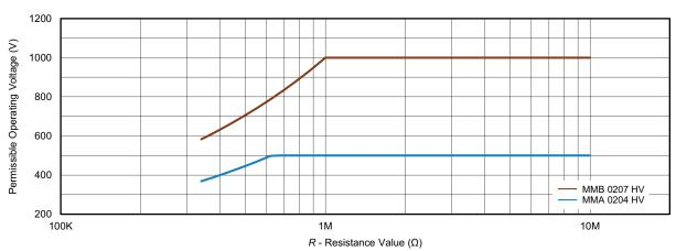
The permissible operating voltage equals the rated voltage  $U_{\rm R} = \sqrt{P_{70}\,x\,R}.$  For ambient temperatures above 70 °C power derating must be considered
