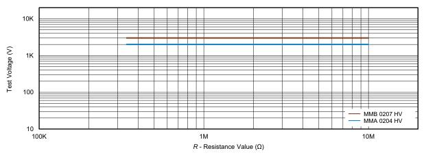
Pulse load rating in accordance with IEC 60115-1, 4.27; 1.2  $\mu$ s/50  $\mu$ s; 5 pulses at 12 s intervals; for permissible resistance change  $\pm$  (0.5 % R + 0.05  $\Omega$ )
