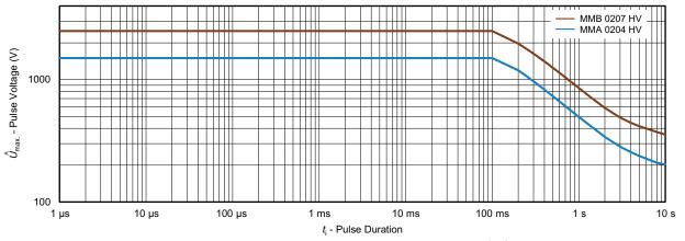
Maximum pulse voltage, single and continuous pulses; applicable if  $\hat{P} \leq \hat{P}_{\text{max}}$ , for permissible resistance change  $\pm$  (0.5 % R + 0.01  $\Omega$ )
