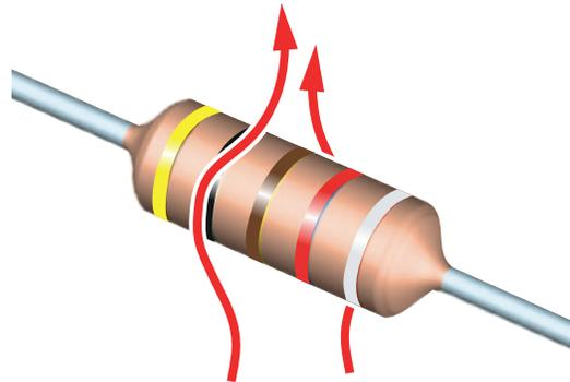
The higher power resistors have larger bodies that improve heat transfer to air, whereas smaller body through-hole parts operating at a lower power have a greater proportion of the power conducted to the PCB. This is indicated by the different points of derating for the different resistor technologies, as illustrated by the graphs below.
