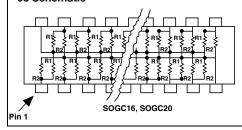
TTL dual-line terminator; pulse squaring, 14 or 18 pairs of resistors
