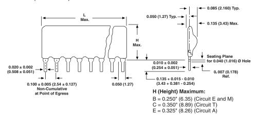
Pin #1 is extreme left-hand terminal on side with marking.
