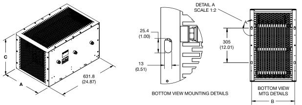
Indoor (IP20) version shown. Outdoor (IP23) version will have a solid elevated roof instead of the screen top shown for the indoor version.
