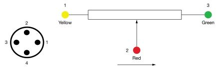
Direction of wiper displacement with shaft extended
