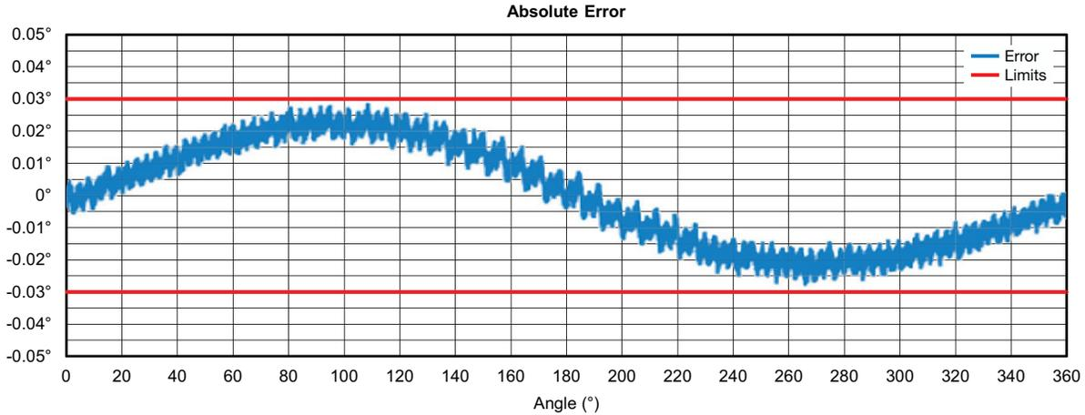
Fig. 6 - Example of runout close to the limit value
