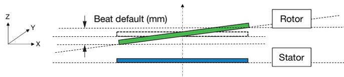
Rotor axis and stator axis are the same but the reference surfaces are not parallel
