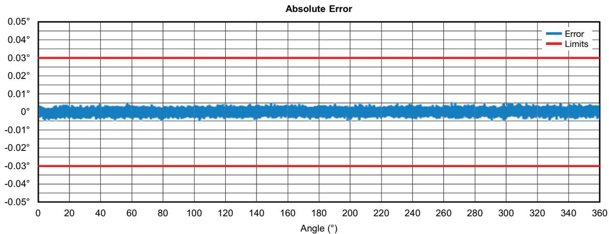
Fig. 5 - Accuracy result without runout
