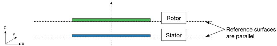
Rotor axis and stator axis are the same → reference surfaces are parallel
