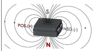
When a positive (+) voltage is placed on the terminal marked with the polarity dot and the opposite terminal is negative (-), the resulting current flow will create a magnetic south pole on the top side of the IHLP.
