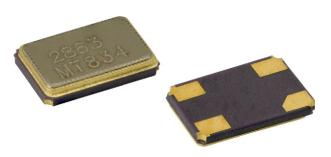
The XT35 is a miniature SMD crystal with 5.0 x 3.2 (mm) ceramic package and a height of 0.8 mm. 12 MHz to 39 MHz frequency makes it widely applied in PDA, GPS, MP3, and portable instruments.
