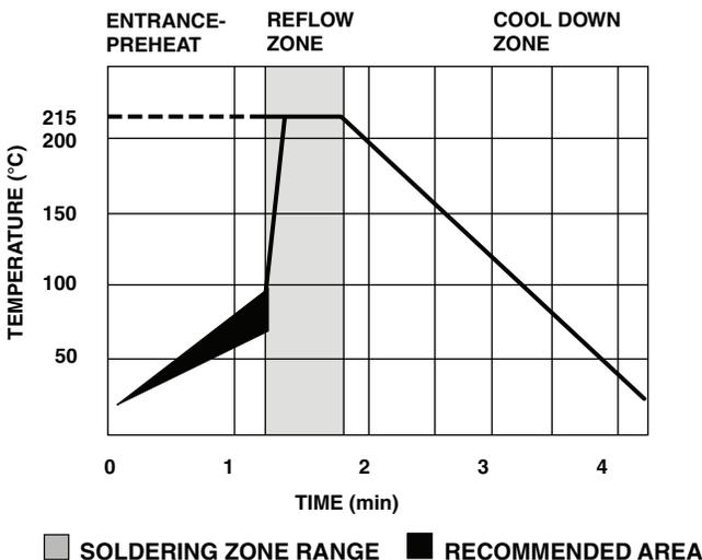
With vapor phase reflow, heat reaches the product uniformly and quickly because of vapor condensation heating. During condensation heating a dense vapor condenses on all exposed surfaces. Due to the inherent low boiling point (+215 °C) for liquids used in vapor phase, ceramic chips can be reflowed without thermal shock damage. Vishay offers the following recommendations:
