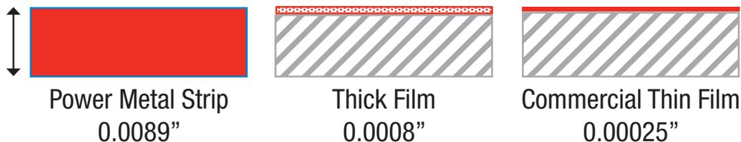
Power Metal Strip resistors are frequently used in applications that experience high-energy, short-term pulse transients:
