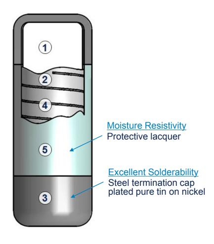
The MELF resistor's contacts are built from steel termination caps, plated with pure matte tin on nickel, and support excellent solderability. The protective lacquer provides the component with superior moisture resistivity, verified according to the 85°C/85 % biased humidity test for 42 days. The UMA 0204, UMB 0207 MELF resistors offer high reliability in harsh operating environments, including high humidity and high temperature.
