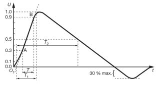
Front time: T<sub>1</sub> = 1.67 x T = 1.2  $\mu$ s ± 30 % Time to half-value: T<sub>2</sub> = 50  $\mu$ s ± 20 %
