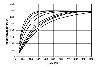
Heating is also function of time according to the formula :  $\Delta QT = \Delta QT \text{ max.} (1 - e - (\underline{t}))$
