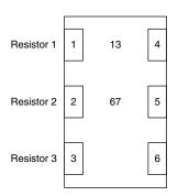
For arrays with 4 to 8 resistors, the marking shall be located adjacent to the first 4 resistors of the array. The first resistor, R1, of the array is on the left hand end of the array whilst reading the marking, as follows:
