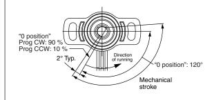
(3) 981 HE D-Shaft Continuous rotation Shaft: Ø 6.35 flatted 16 mm FMF Model: 981HE-0-x-x-W-x-1F16
