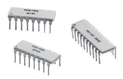
A dual-in-line monolithic ceramic package in a variety of sizes and configurations. A rugged, low cost packaging technique with 4 leads to 20 leads that allows higher resistance integration than chip and wire ceramic packages.
