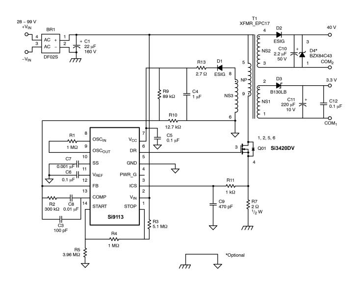
FIGURE 3. Dual Output Flyback Converter with Moderately Regulated Outputs (As used on Demo Board DB-2)
