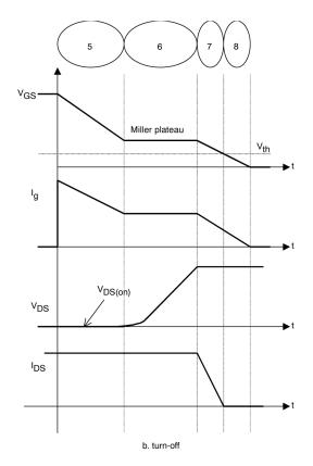
FIGURE 2. Switching waveforms for a typical MOSFET in a buck converter
