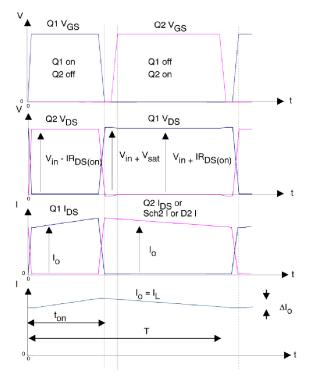
FIGURE 8. Current and voltage waveforms for the buck converter in constant-current operation
