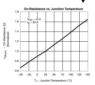
FIGURE 9. Normalized r<sub>DS(on)</sub> versus temperature for a typical device
