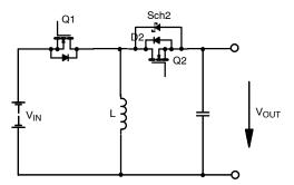
FIGURE 15. Basic circuit schematic for the buck-boost converter
