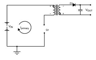
FIGURE 19. Schematic showing turn-on of Q1
