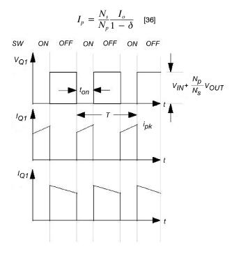
FIGURE 22. Current and voltage waveforms for a flyback converter in continuous mode
