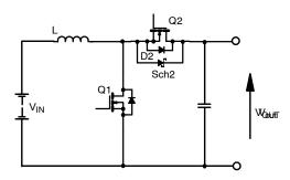
FIGURE 11. Basic circuit schematic for a boost converter
