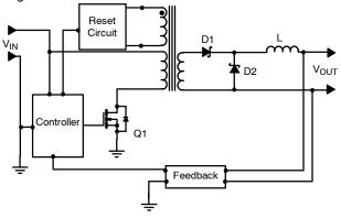
FIGURE 23. Schematic of an isolated forward converter
