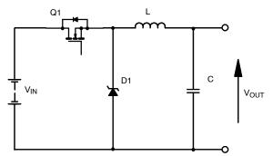
FIGURE 1. Typical circuit of a buck converter
