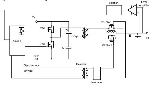
FIGURE 27. Schematic of a half-bridge converter
