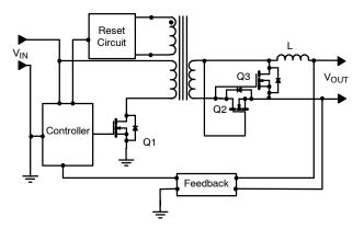
FIGURE 25. Self-driven synchronous rectification in a forward converter
