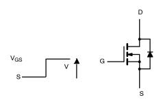
FIGURE 3. Schematic of an n-channel MOSFET
