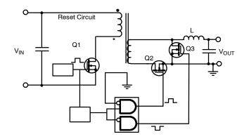
FIGURE 26. Synchronous rectification in a forward converter using a discrete driver
