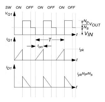
FIGURE 21. Current and voltage waveforms for a flyback converter in discontinuous mode
