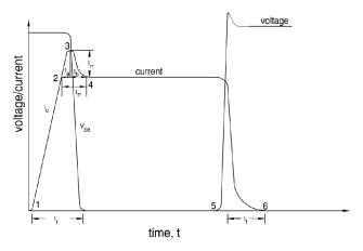
FIGURE 10. Idealized switching waveform for a MOSFET
