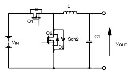
FIGURE 5. Basic circuit schematic for a buck converter
