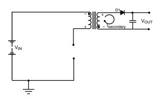
FIGURE 20. Schematic showing turn-off of Q1
